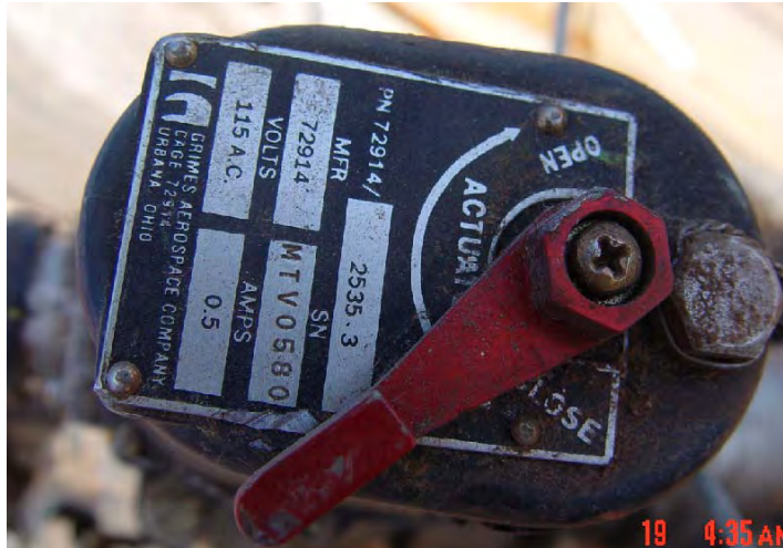
Photo - Forward Outflow Valve
